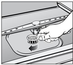
■ Return the combination filter so that it lies flat in the base of the dishwasher. Secure it by turning the handle clockwise.
